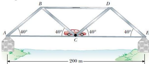
52. A bridge truss extends 100m across a river (Fig). The structure is free to slide horizontally to permit thermal expansion. The structural components are connected by pin joints, and the masses of the bars are small compared with the mass of a 1500kg car halfway between points A and C. Show that the weight of the car is in effect equally distributed between points A and C. Specify whether each structural component is under tension or compression and find the force in each.
