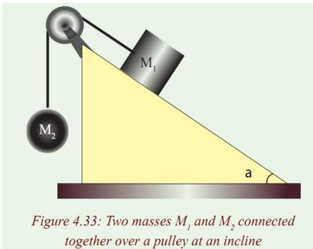
Figure 4.33: Two masses  $M_1$  and  $M_2$  connected together over a pulley at an incline
