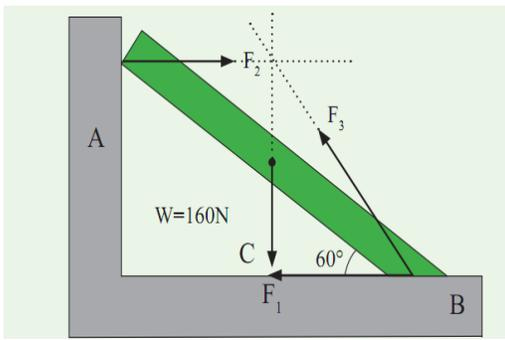
The coefficient of static friction between the ladder and the ground is 0.53. How far up the ladder can the firefighter go before the ladder starts to slip?
